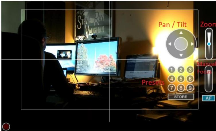
5. Initially there will *not* be a blue dot in any of the controls, move your mouse over to the Pan/Tilt control area, and then left click hold. You will now have a “Joystick” type control of the AVer camera.
